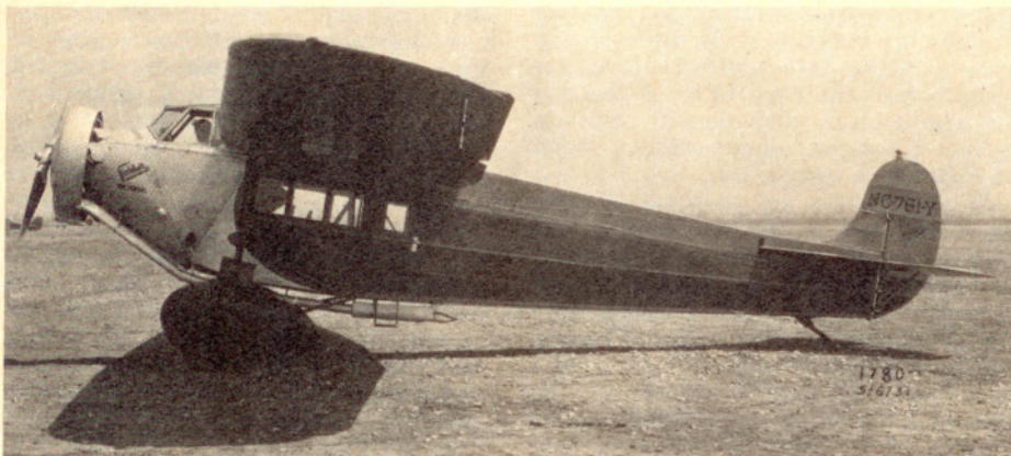
One of the last Universals, photographed at the factory in May 1931. Note the enclosed pilot's cabin, increased passenger window area, and improved streamlining.
